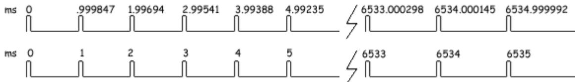
The first line illustrated the real time at which timer management occurs. The second line is the time at which the kernel expects the timer to be fired.
