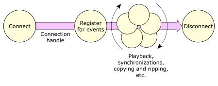
Client application workflow with MME from connection to disconnection
