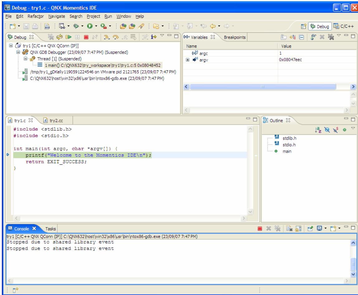
12. To step to the next line, click on the toolbar. (This would typically be F10 in VC++.) If the next line were a function that you wanted to *step into* you would have clicked . (This would typically be F11 in VC++.)
