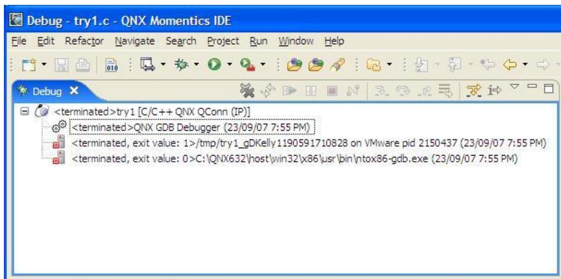
At this point, the program on the target has run to normal completion (second line) as well as the debugger component on Windows (third line). If you click
