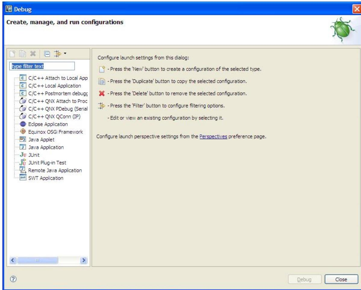
A configuration is required to build an association between a project, its executable and the target on which it will run and be debugged. Such an association is called a “Run Configuration”.
